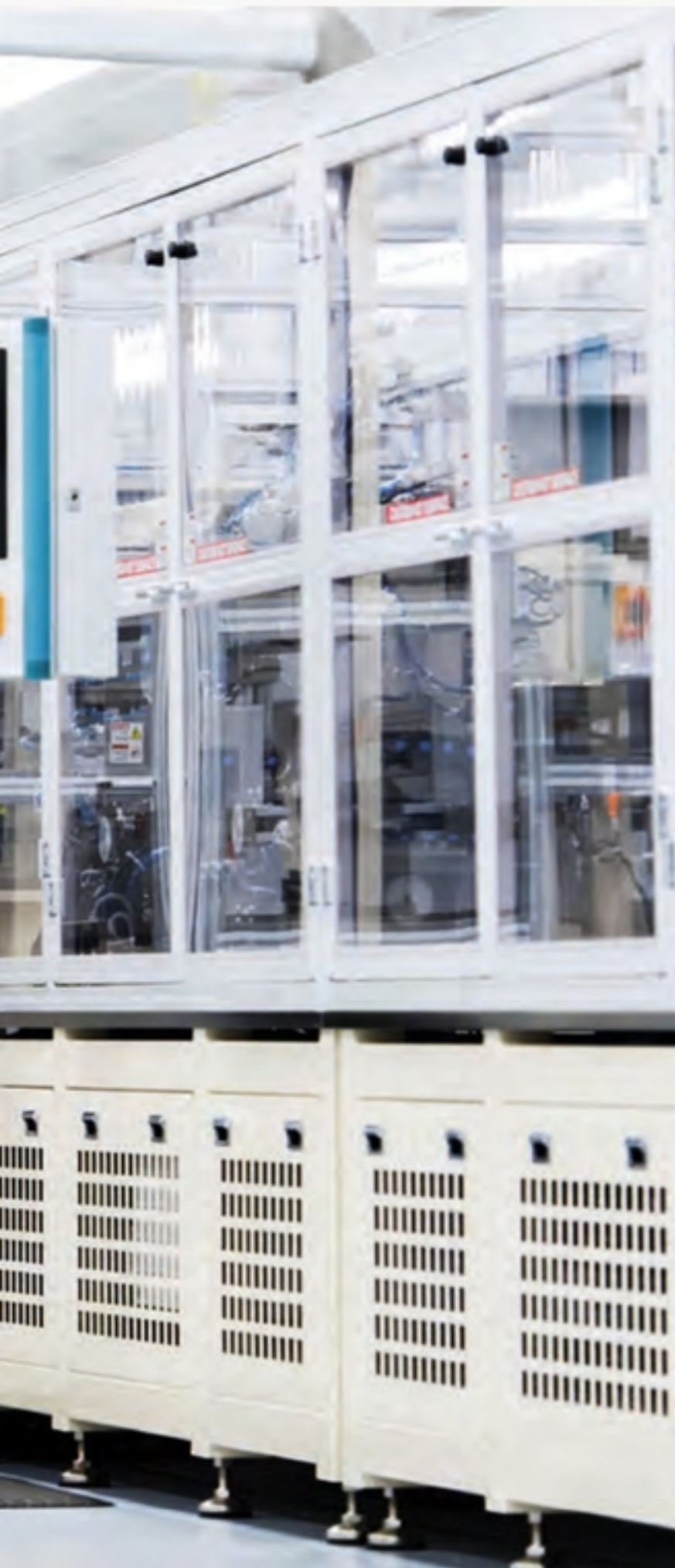
Xalt batteries (above) achieve an impressively high cycle rate thanks partly to the supplier's ultra-clean manufacturing processes that see the cells being built in highly controlled environments (below). As a result, the first time that the electrode and cathode come together is during assembly, and they're not touched by human hands until inspection
